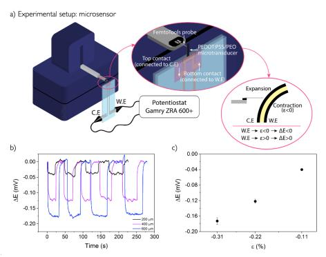
**Figure 3.** Sensor characterizations of a 2900 x 250 x 23  $\mu$ m microbeams: (a) schematic representation of the experiment setup, (b) output voltage response to a mechanical stimulation of 200, 400 and 600  $\mu$ m, (c) OCV response as a function of applied strain.
